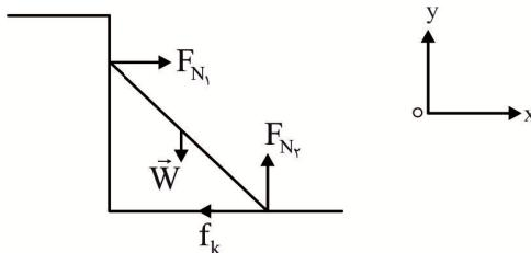
$$\begin{cases} F_{net_x} = 0 \rightarrow f_k = F_{N1} = 100\text{ N} \\ F_{net_y} = 0 \rightarrow F_{N2} = W = 240\text{ N} \end{cases} \rightarrow R = \sqrt{f_k^2 + F_{N2}^2} \rightarrow R = \sqrt{100^2 + 240^2} = 260\text{ N}$$
